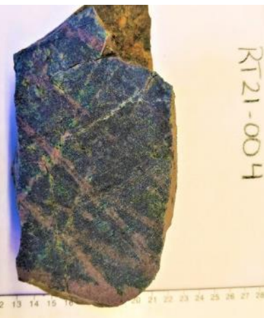
Porphyry-related stockwork pink quartz veins with magnetite and minor chalcopyrite (bornite) in chlorite-magnetite alteration of Jurassic Bonanza Fm. volcanics
